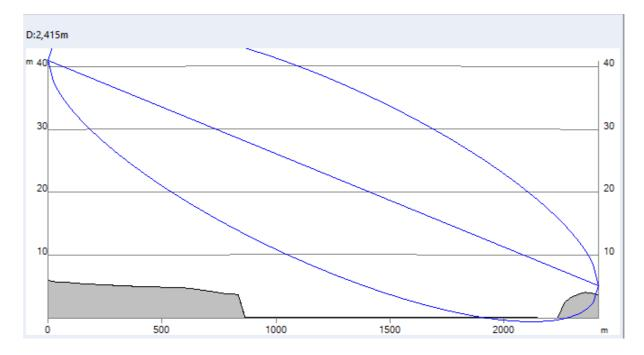
The image above shows the terrain profile from *BALLINA Telstra Exchange* to the site based on the SRTM digital elevation model. The distance between the two points is *nearly 2.4 km*, and *both* LOS and First Fresnel Zone are *nearly clear*. Therefore, service reliability from it should be *high*.
