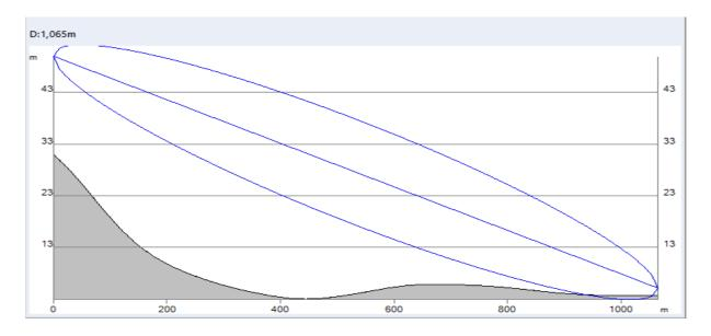
The image above shows the terrain profile from *Suvla Street BALLINA* to the site based on the SRTM digital elevation model. The distance between the two poits is *almost 1.06 km*, and *both* LOS and First Fresnel Zone are nearly clear. Therefore, service reliability from it should be *high*.
