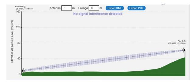
Assuming there is no non-terrain obstruction, and the predicted signal strength is close to the reality from station at *Suvla Street BALLINA*, the receiving antenna is recommended to be raised to 5 m AGL in this setup to achieve *a clearer First Fresnel Zone*, and *then a better* connection can be attained.
